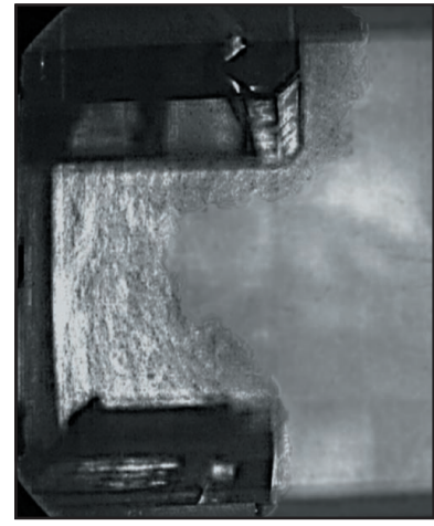
Schlieren image showing spillage at 3375 cfm total exhaust and 2100 cfm (62%) makeup air supplied internally. Spillage began at about 25% makeup air.
